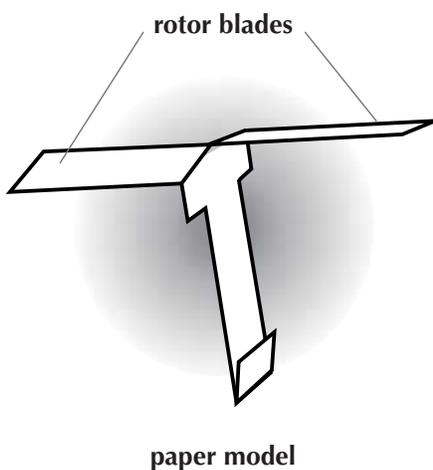
Lift is produced by the pressure differences caused by the shape of rotating blades; this is the same way lift is produced by aircraft wings. The rapidly moving air over the top of the blade creates low pressure; the air beneath the blade is moving slower, so it creates higher pressure (see "Paper Bag Mask" pages 26-27, Bernoulli's principle, for more information). High pressure under the rotor blades creates lift which causes the aircraft to rise.
