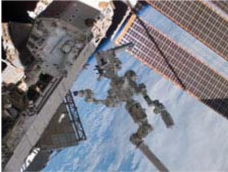
Dextre is attached to the end of the International Space Station's robotic arm, Canadarm2. Image Credit: NASA
