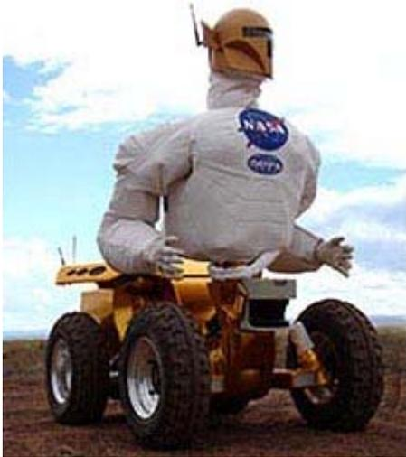
Robonaut could perform tasks that astronauts otherwise would have to do. Image Credit: NASA
